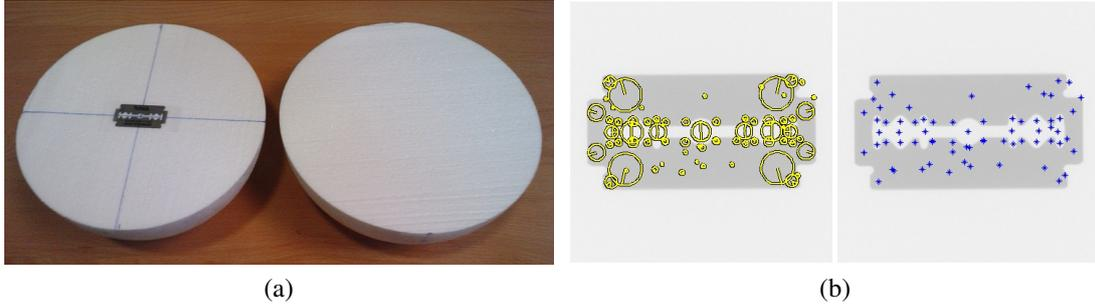
Figure 9: Characterization of a razor blade, a) sphere of EPS (*Expanded PolyStyrene*), and b) razor blade with two SIFT representations: magnitude-orientation, and keypoints.
